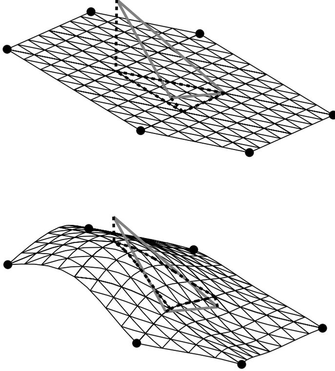
Figure 7: Top: original surface and a surface attractor. Bottom: resulting constrained variational surface.
