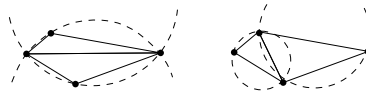
Figure 1: An illegal edge has a triangle whose circumcircle contains the opposite vertex of a neighboring triangle (left). By reconnecting (‘flipping’) the edge, the circumcircles become disjoint (right).
