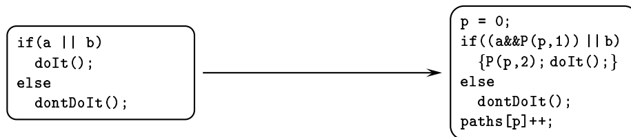
Fig. 4. Instrumentation for Path Profiling. The right box shows how the code segment on the left has been modified to count how many times each path is executed.
