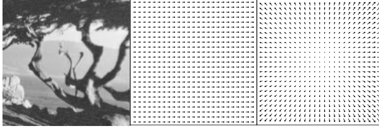
Figure 5: Textured plane and vector field for translation (TTS) and divergence (DTS).
