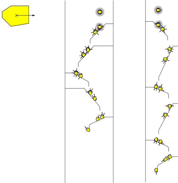
Figure 5: An optimal design of five fences, and a design of six alternating fences allowing for a narrower belt. Every line segment emanating from the part represents a possible orientation of the part.
