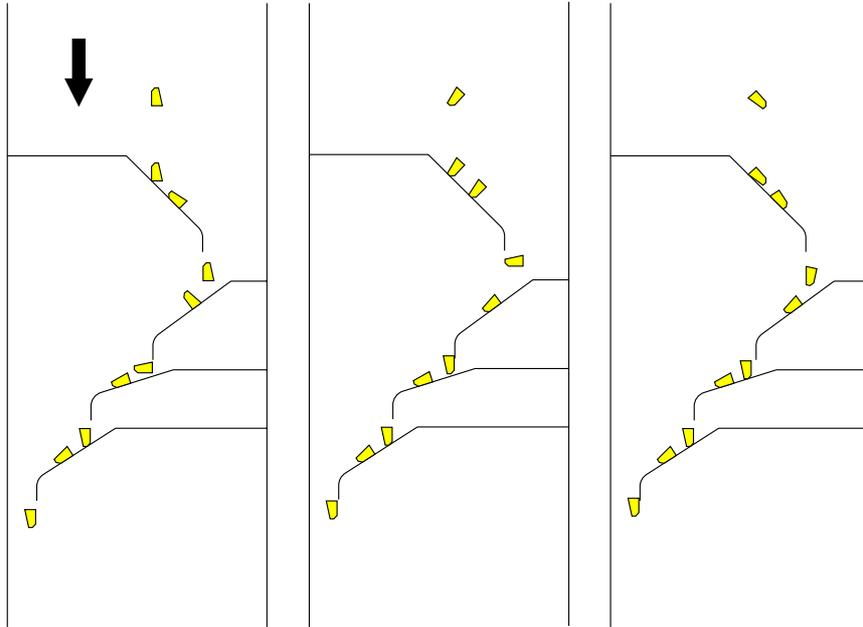
Figure 1: Three overhead views of the same conveyor belt and fence design. The traversals for three different initial orientations of the same part are displayed. The traversals show that the part ends up in the same orientation in each of the three cases.
