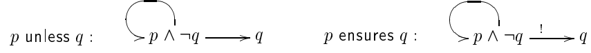
Figure 4: unless and ensures. The predicates p \wedge \neg q and q define sets of states. The arrows depict possible transitions between the two sets of states. The arrow marked with ! is a guaranteed transition.
