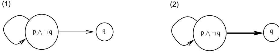
Figure 6: (1) is {}_P \vdash p unless q and (2) is {}_P \vdash p ensures q . The thick line means a guaranteed transition.
