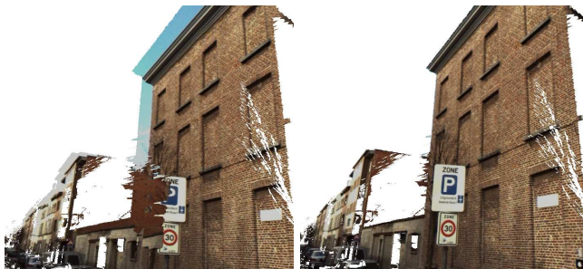
Fig. 1. Part of a panorama projected onto the triangle mesh generated from a LiDAR point cloud, before and after registration.
