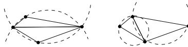
Fig. 1. An illegal edge has a triangle whose circumcircle contains the opposite vertex of a neighboring triangle (left). By reconnecting (‘flipping’) the edge, the circumcircles become disjoint (right).
