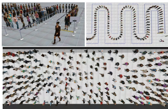
Figure 12: Two application scenarios. First one is a pure 1D-traffic situation where virtual walkers are queuing along a winding path (top). Second one is a corridor traffic that combines avoidance and following behaviors (bottom)
