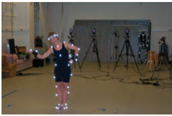
Figure 2: A subject wearing retro-reflective markers in the motion capture laboratory.
