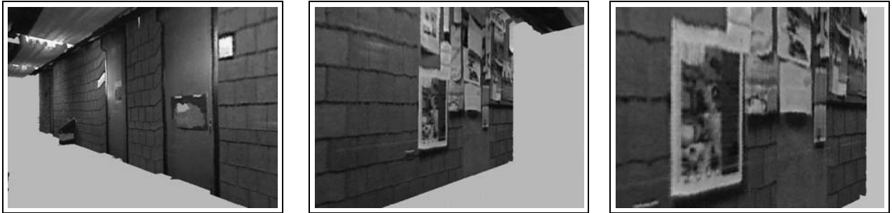
Figure 11: 3D Model generated (a) from raw sensor data, and (b) using our algorithm, in which 94.6% of all measurements are explained by 7 surfaces. Notice that the model in (b) is much smoother and appears to be more accurate.
